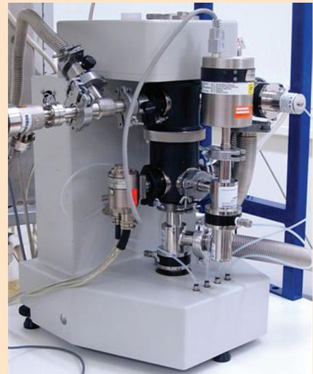
Primary vacuum standard based on conical piston technology.
