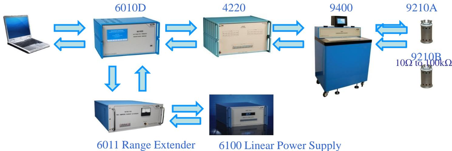
The 6010D bridge is extensively used in NMIs and industry for resistor maintenance and to calibrate customers resistors in the range of 1Ω to 100kΩ
